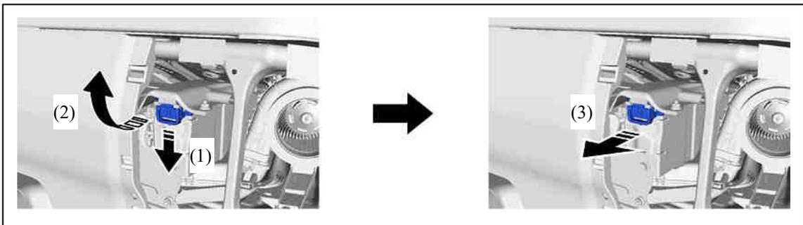
5. Carry the removed service plug grip in your pocket to prevent other staff from accidentally reinstalling it while you are dismantling the vehicle.
