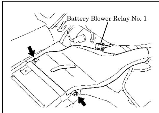
16 Remove battery bracket reinforcement.
