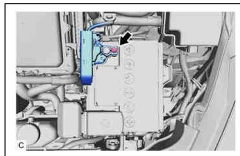
(2) Disengage the 2 claws and open the battery terminal cap.
