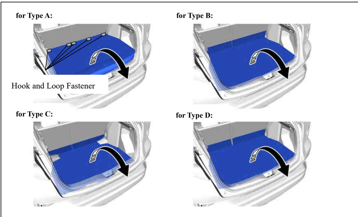
2. Remove battery service hole cover assembly.
