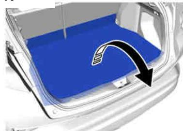
3. REMOVE BATTERY SERVICE HOLE COVER ASSEMBLY (for M20A-FXS, w/o Spare Tire)
