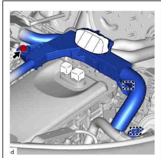
8. DISCONNECT ENGINE WIRE (for M20A-FXS, M20B-FXS, M20F-FXS, M20G-FXS)
