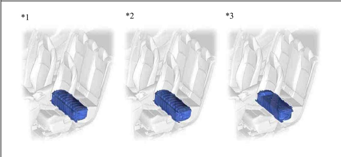
HV Battery Pack Mounted in Cabin Area
