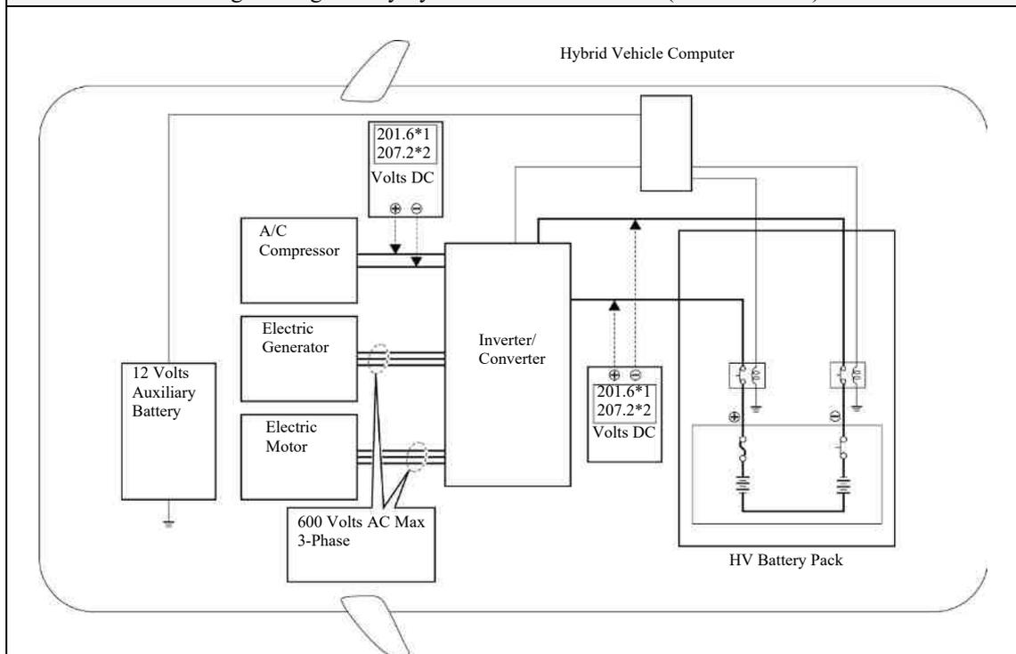
High Voltage Safety System – Vehicle On and Operational (**READY-ON**)
